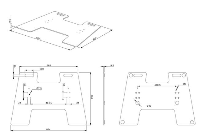
Neomounts Measuring unit: mm
